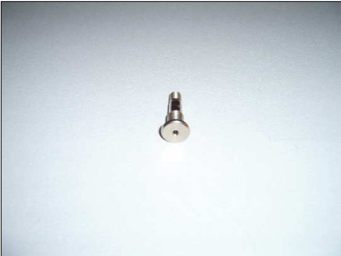
The bottom of the stem before cutting air passages.
