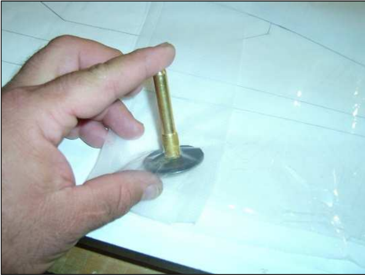
Stem pushed through the hole in the bag.
